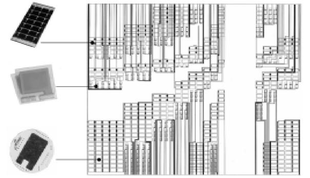
SmartWrap elevation showing thin-film photovoltaics, organic light-emitting diodes, and thin-film batteries. Image by KieranTimberlake Associates
